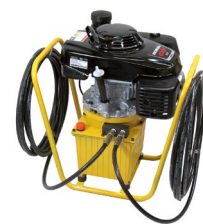
4-stroke motor (3 kW), Honda
