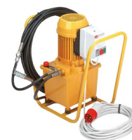
Three-phase motor (1.5 kW, 230/380 V)
