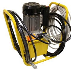
Alternating current motor (1.5 kW, 230 V)
