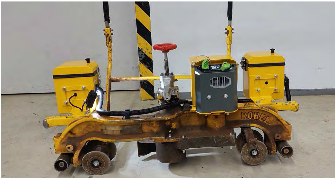
Fig. 7-1 attached Power Unit GPU 3400 +S to Robel 13.44/13.45
