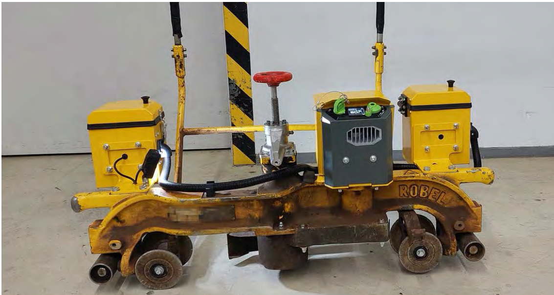
Fig. 3-2 installed Power Unit GPU 3400 +S on Robel 13.44/13.45
